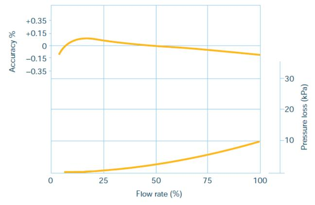
Figure 1 – M1AR and M2AR Accuracy and Pressure Loss
