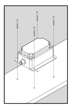
Figure 6 - Mounting the FFM100
