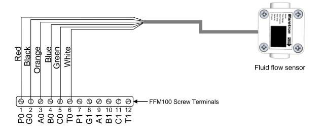
Figure 8 – Fluid flow sensor Connection Diagram
