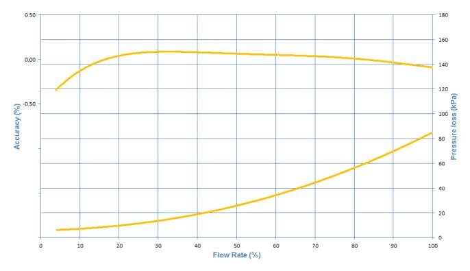
Figure 3 – M8AR and M16AR Typical Accuracy and Pressure Loss
