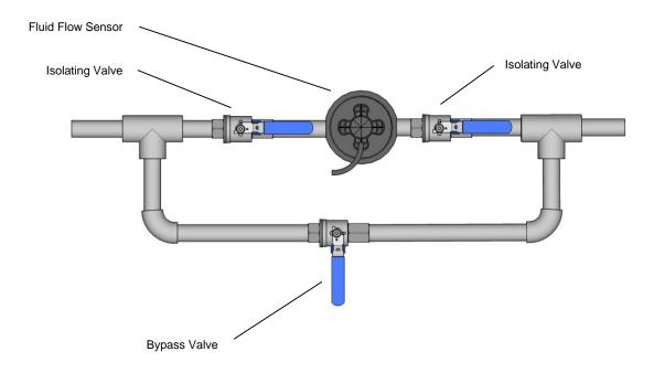
Figure 7 – Fluid Flow Sensor Installation with Bypass and Isolating Valves
