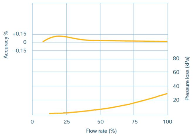
Figure 2 – M4AR Typical Accuracy and Pressure Loss
