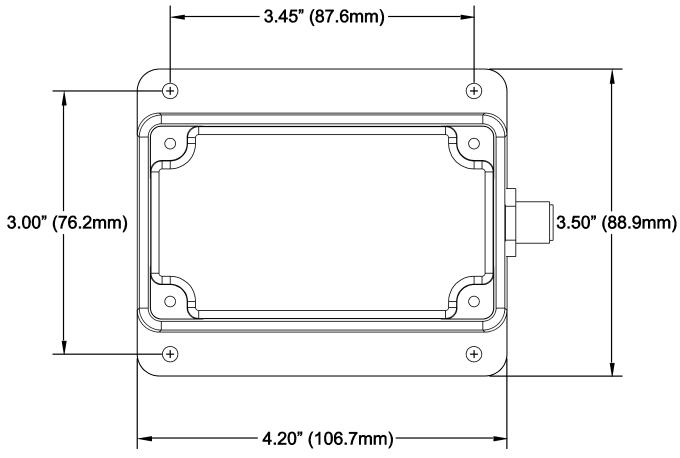
Figure 11 - Mounting Surface Template
